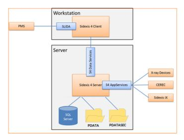
**Example 2:** two IT networks – one for your PMS and one for all components of the Sidexis 4 system and the X-ray components
